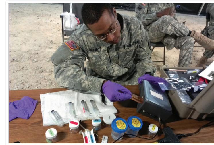
2LT Hays tests water samples during CA (Customer Assessment) of the prototype Environmental Sentinel Biomonitor system.
