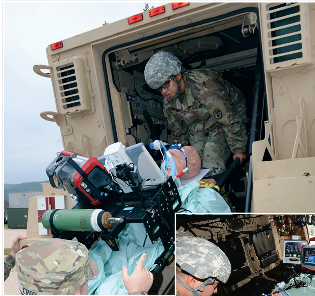
Attached to a simulated patient's litter, the IPRT device is maneuvered into a field ambulance and secured.
